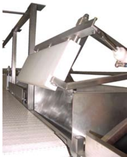
Completely wash down compatible, including movable panels for easy cleaning
