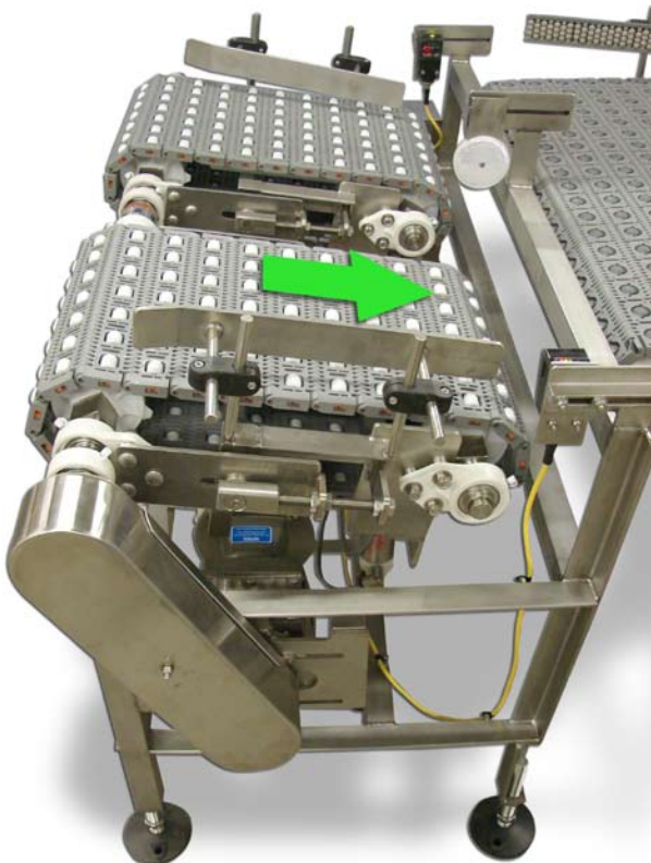
Dual line indexing conveyors for dual convergence
