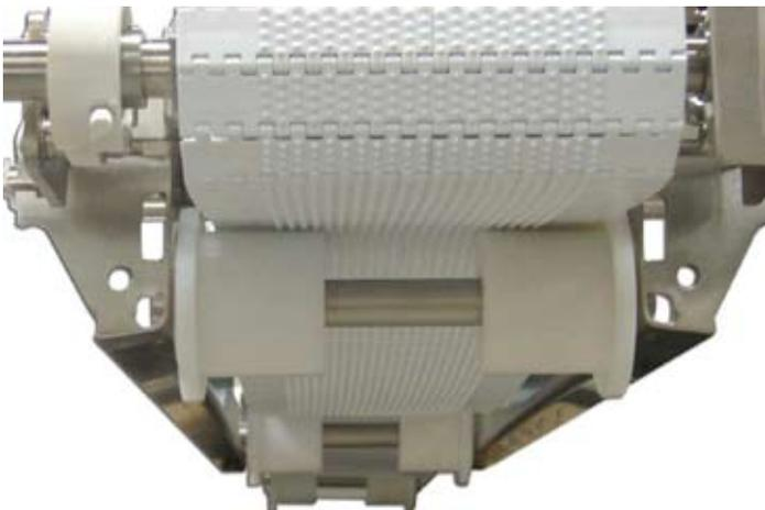
Open access to the underside of the conveyor ensures you are able to clean all areas. Roller shaft is easily removable from the frame for thorough cleaning.
