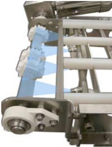
Optional clean-in-place nozzles permits automatic cleaning while belt is running. Simply open a water valve!
