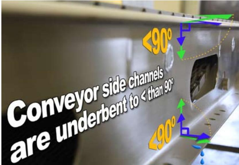
Vande Berg Scales makes a highly reliable food-grade (sanitary) conveyor that is easy to clean. Side channels are under-bent to less than 90-degrees resulting in less water accumulating on the conveyor after washdown.
