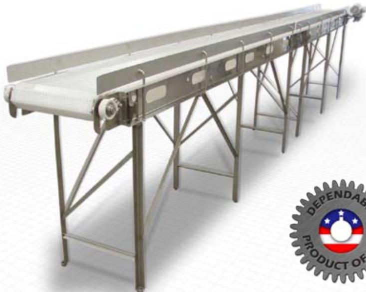
Easy-to-Clean conveyor with an open frame design. The openings along the belting frame permit access to the undersides of the belt. The cross bracing support underneath the conveyor is rotated to eliminate standing water.
