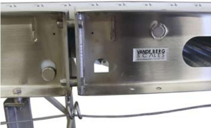
Our design accommodates 20-60 foot conveyors by creating multiple identical 10-foot sections. This keeps costs down.
