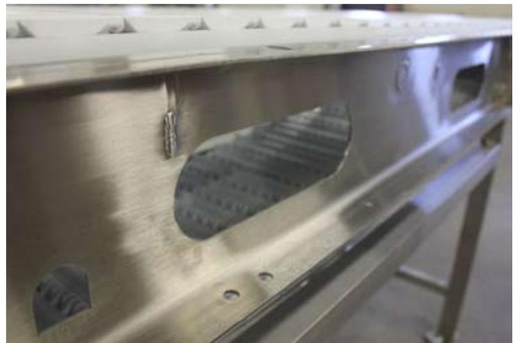
Open access points on the sides of our conveyor allow for easy cleanability for wash down applications.
