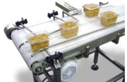
Line convergers combine multiple lines to single lines
