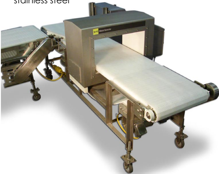
High-profile metal detector with wide conveyor belt - useful for scanning large parcels.
