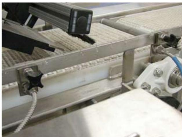
*Brackets ensure proper placement of photo eyes*
