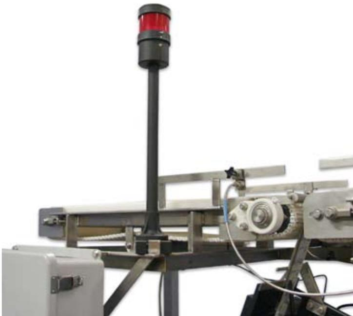
*Low label warning lights save time and labor, making label changing fast and efficient*
