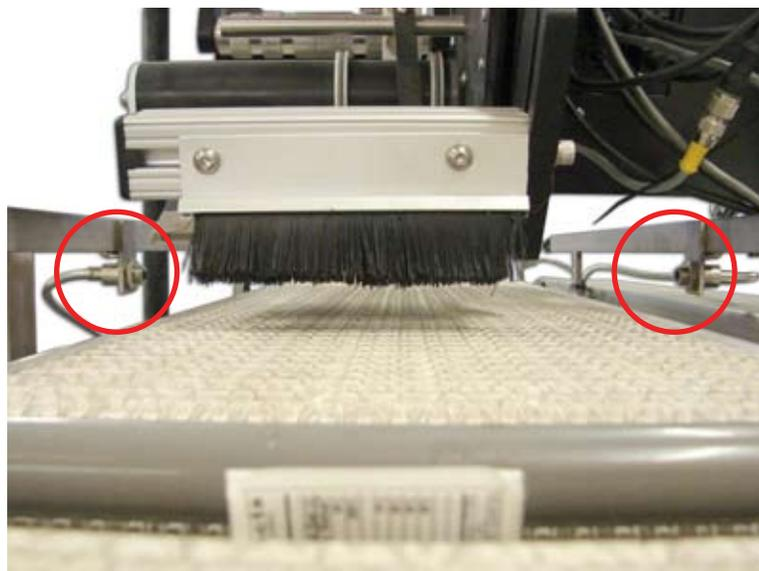
*Photo eyes are triggered when product passes, telling the labeler when to apply the label*
